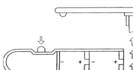
Open the battery compartment and insert 2 x AAA batteries respecting the polarity.
