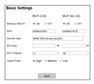
**Wi-Fi Channel:** Set the channel to a value that puts this wireless network at least four channels apart from an existing wireless network that might be in close proximity. For example, if another 2.4 GHz wireless network in range is set to channel 2, then it'd be best to set your Intellinet Access Point to channel 6 or higher.
