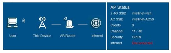
If you create a repeater or WISP setup, this display can be very helpful in determining whether or not the connection succeeded. The example below shows an unsuccessful repeater connection. The status continues to show 'Scanning ...' and Internet displays as 'Disconnected'.
