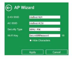
Default values for Access Point (AP) mode, if device is <u>not</u> connected to a router or DHCP server with the LAN port.
