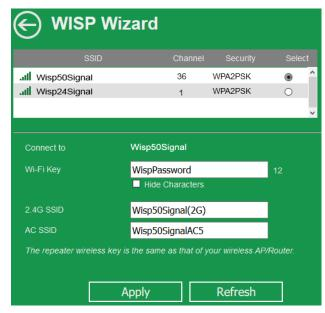
Note: The wireless encryption key for your clients is the same as the encryption key of the WISP network.
