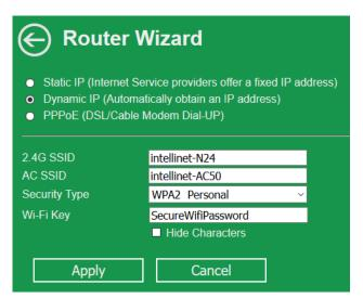
Click 'Apply' to activate the settings. The Access Point will then perform a reboot. After this, you can re-connect to the admin web interface, and from there you have access to advanced wireless settings.
