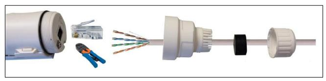
Use a Cat5e or Cat6 installation cable and thread it through the two plastic covers and the black rubber seal. Then use a crimp tool to affix an RJ45 plug to the cable.
