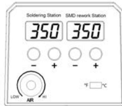
1. Press the button "+" or "-" to adjust the temperature. In short press, the set-point will change  $\pm 1^\circ\text{C}$ . In long press, the set-point will change quickly and reach your target temperature.
