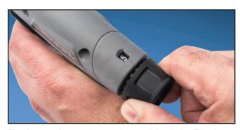
To change the tension setting, pull back the Tension Adjustment Knob, match it to the appropriate cable tie cross section tension setting, and disengage the knob.
