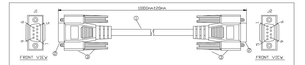
I.CABLE:NO UL.,28AWG(7/0.127),TINNED AND STRANDED COPPER WIRE INSULATOR:PVC,ID:0.85mm ,CABLING:9C+DRAIN WIRE SHIELD:AL/MY COVERAGE
