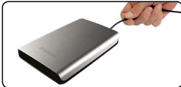
1. Connect the interface cable to Verbatim Store 'n' Go Portable Hard Drive.
